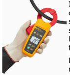
If we occasionally need to check the battery voltage or the charging current, we simply use a portable clamp-meter, which is supplied with each kit for free. Charging current is measured by simply putting the clamp around a positive or negative wire to the battery. To work out the power, the current is then multiplied with the battery volts.
