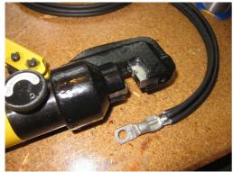
This is a very important part of the jigsaw puzzle and if not done right, can cause losses and heat build up which could even lead to fire. We have seen too many connections oxidise and burn out to trust "off the shelf" connectors.
