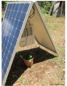
Making a couple of litres of water from the air even on the driest of days is easily done with as little as one A-Frame panel set-up, a battery, a small inverter and a compressor dehydrator.
