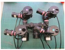
**To avoid any solar energy waste,** multiple water proof, high quality, food grade brushless micro pumps are assembled in series or parallel to meet the exact
