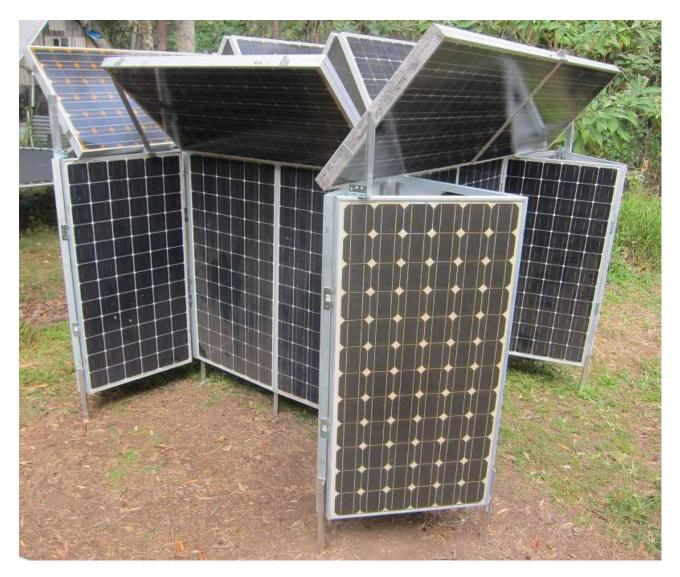
**It is made up of 36 x 195W panels in parallel,** charging 24V 320Ah batteries made up of 8 x 6V 160Ah Maxon Electric Vehicle batteries coupled with a super capacitor.
